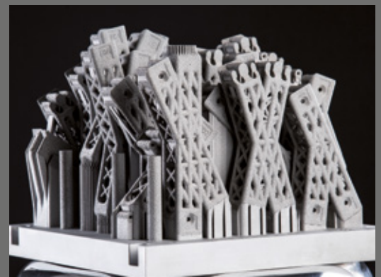
Picture 4 Assembly parts of the partition after 3D process
